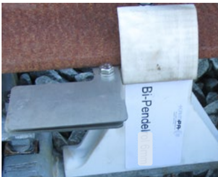
Figure 7: Feeler gauge for measuring and adjusting the pendulum in case the switch rail has a vertical shear ('cat's back')
