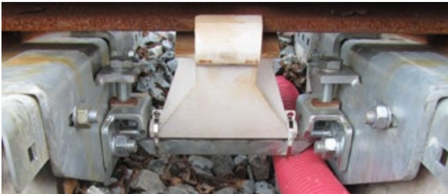
Figure 8: DeltaSwitch with adjacent switch rail (top) and lowered switch rail (below).
